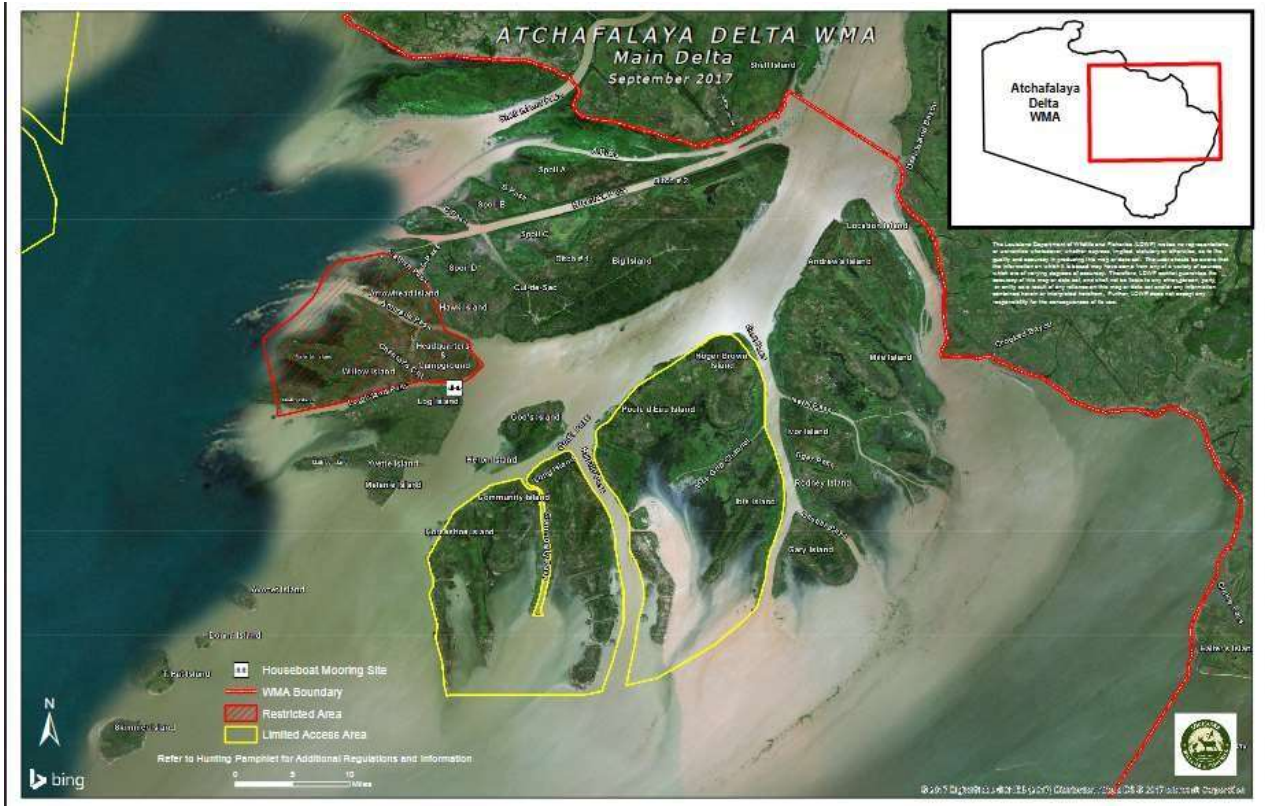
Figure 8. Mouth of Atchafalaya River (top of figure) and the Atchafalaya Delta. Note the narrow shallow finger distributary channels and the wide deep main channel cutting through the delta. The latter is a dredged feature.
