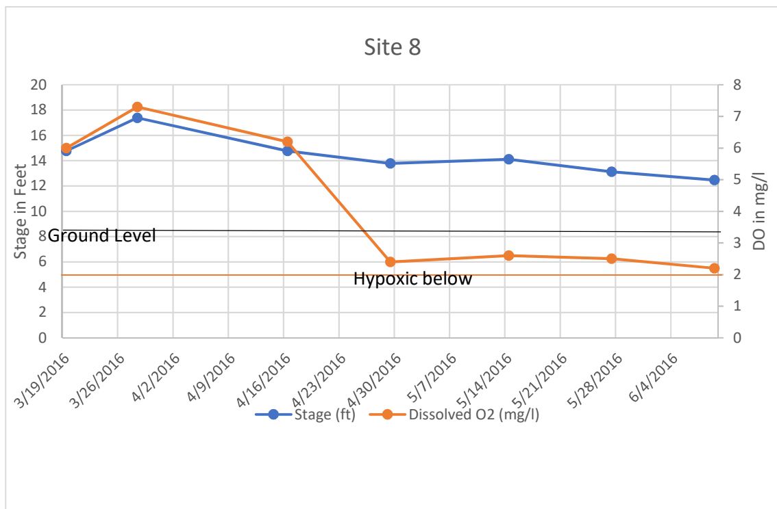
Figure 12. Plot of data from Kong (2017) of stage and DO over the time data as was collected for Site 8. See Figure 7 for comparison.
